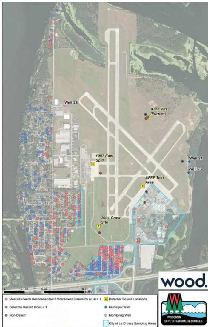
Figure 5. Drinking water test results on French Island in the Town of Campbell. The red circles indicate wells with concentrations above health-based recommendations.
