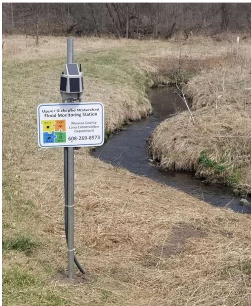
A flood monitoring station in Monroe County [10]
